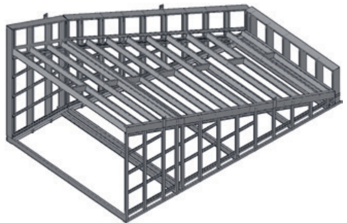
Figure 10 Light steel roof module with integrated parapet (Image courtesy of Ayrshire Framing)
